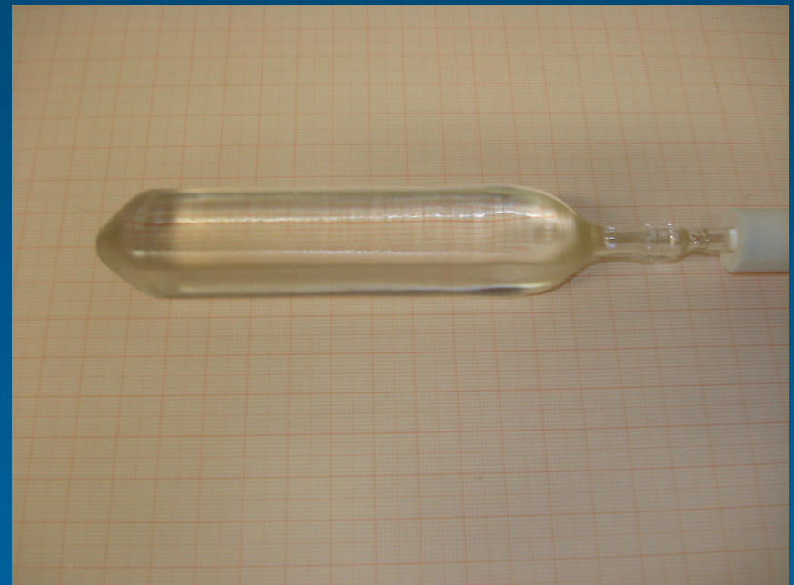
Crystal grown under 99% Ar, 1% O_2 atmosphere
