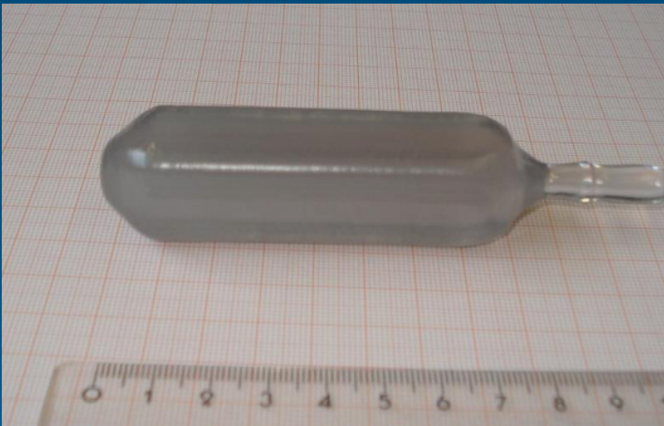
Crystal grown under pure N_2 atmosphere
