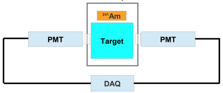
Temperature of target crystal can be varied down to ~1.7 K, while PMTs are operated at room temperature.
