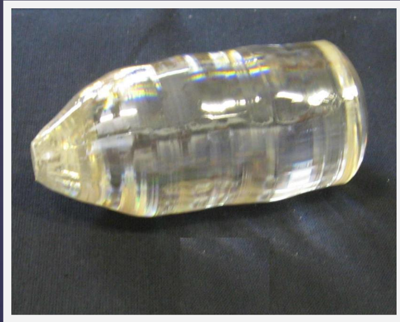
Large volume \text{ZnWO}_4 crystal scintillators up to \text{Ø}50 \times 130 mm
