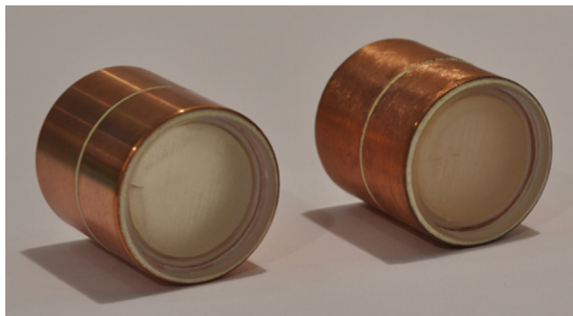
Fig. 1. The enriched 7 LiI(Eu) crystal scintillators. (For interpretation of the references to color in this figure caption, the reader is referred to the web version of this paper.)
