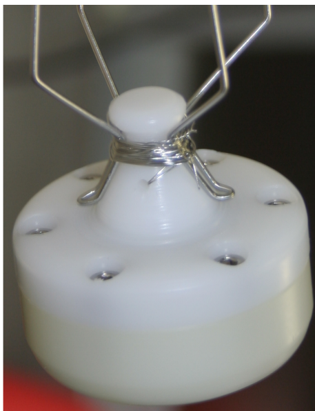
Figure 11. Photo of the encapsulation in which the Borexino ^{241}\text{Am}^9\text{Be} neutron source was placed. Note that the neck contains the same mounting features as the regular source vials.
