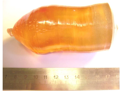
Fig. 6. \text{ZnMoO}_4 single crystal of \varnothing 44 \times 100 mm size grown by Czochralski method.
