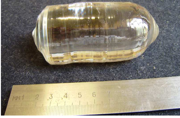
Fig. 1. \text{ZnWO}_4 single crystal of \varnothing 50 \times 100 mm size grown by the Czochralski method.
