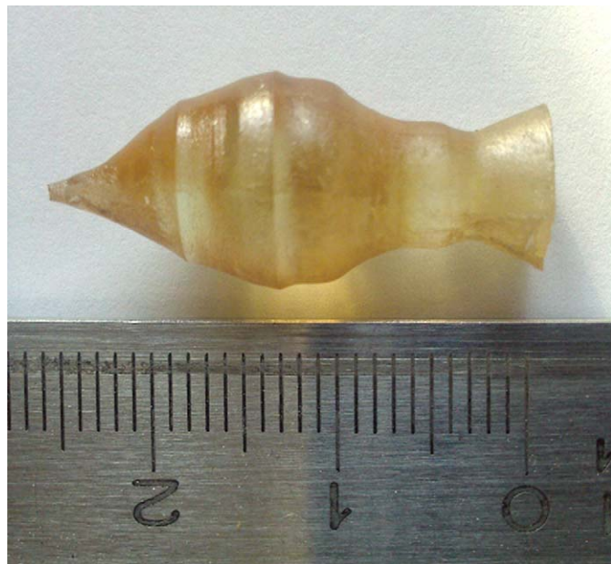
Fig. 1. Produced \text{MgWO}_4 single crystal. The scale is in centimeters.
