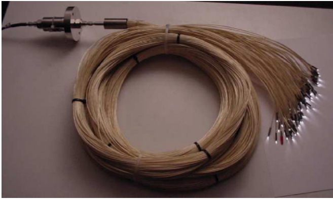
Fig. 15. A bundle of 90 fibers connected to the feed-through and illuminated.
