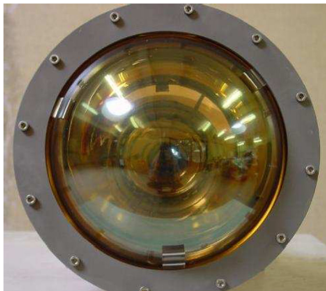
Fig. 13. Sketch of the encapsulation of the outer detector PMTs (top) and a front picture of an encapsulated PMT (bottom).
