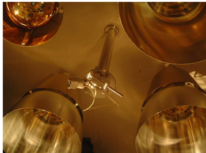
Fig. 20. The pointing device for the oblique type of feed-through: the photo shows a module already installed on the Borexino Stainless Steel Sphere and surrounded by PMTs. The device is designed to point laser light at an angle towards a specific target phototube. The angle is chosen so that the light crosses only the buffer liquid and not the active scintillator.
