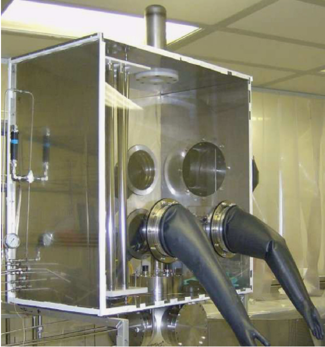
Fig. 21. The glove box used for source insertion. Some of the insertion rods are visible at the left of the glove box.
