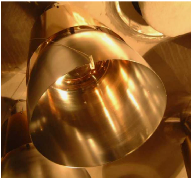
Fig. 16. A picture of an installed photomultiplier: it shows the optical fiber used for timing and charge calibration and the Teflon support attached to the light concentrator.
