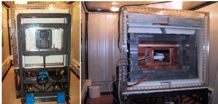
Fig. 6. View of the shield of the R&D installation: closed (left) and open (right).
