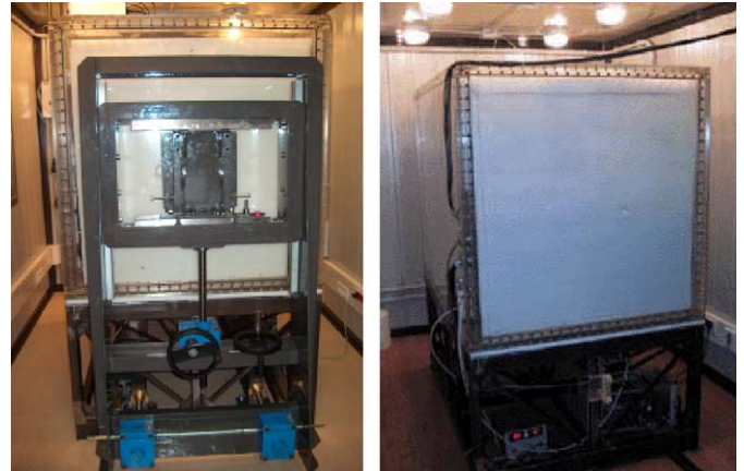
Fig. 2. Shield of the DAMA/R&D set-up and the automatic system to close it.
